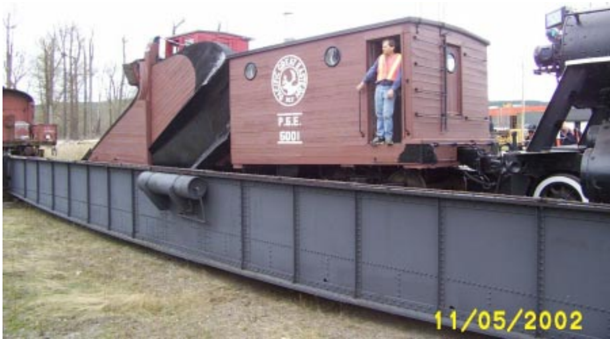
Russell snowplow is eased onto the turntable. Don Holzworth supervising the operation from the doorway of the plow.
